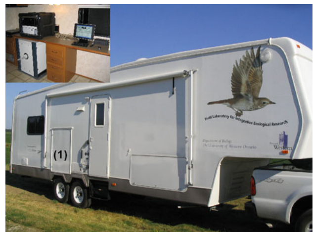
Fig. 1 Mobile laboratory trailer used to transport and operate the Echo-MRI-B quantitative magnetic resonance body composition analyzer. The magnet unit of the QMR analyzer can be loaded into the trailer through an exterior hatch (1) and bolted to the frame of the trailer. Inset the interior of the laboratory with the QMR magnet under counter and electronics/computer above
